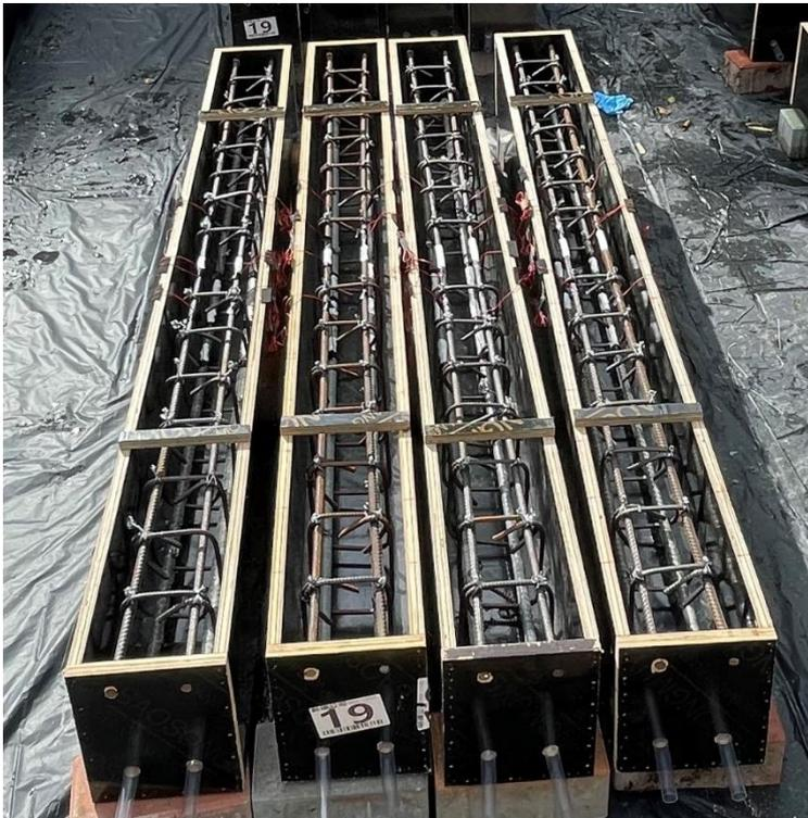
Figure 7.2 Framework of FCSR beam
