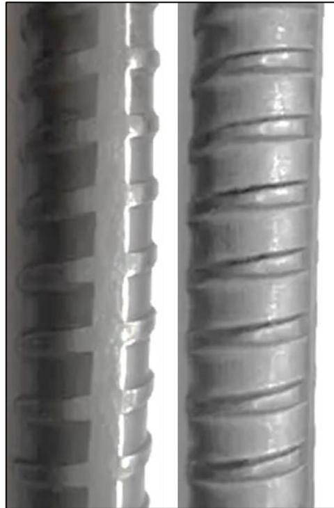
(b) Screw-thread steel rebars
