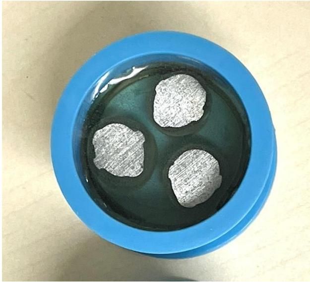
Figure 5.4 Cold mounting of specimens in a plastic mould
