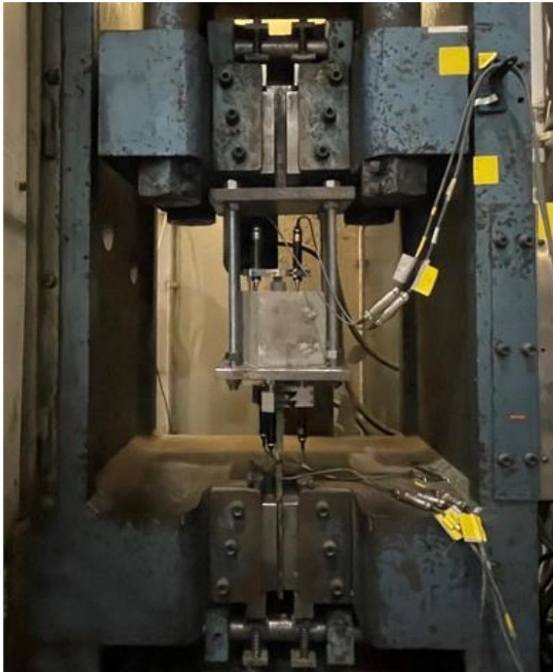
Figure 6.4 Setup for pull-out tests
