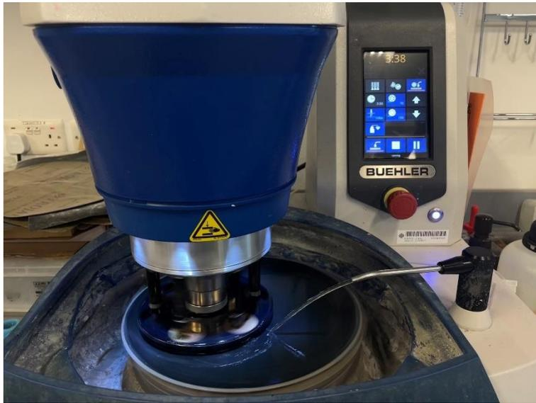
Figure 5.5 Polishing the observation surface of cold-mounted specimens
