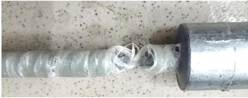
(a) A failed FCSR under tension
