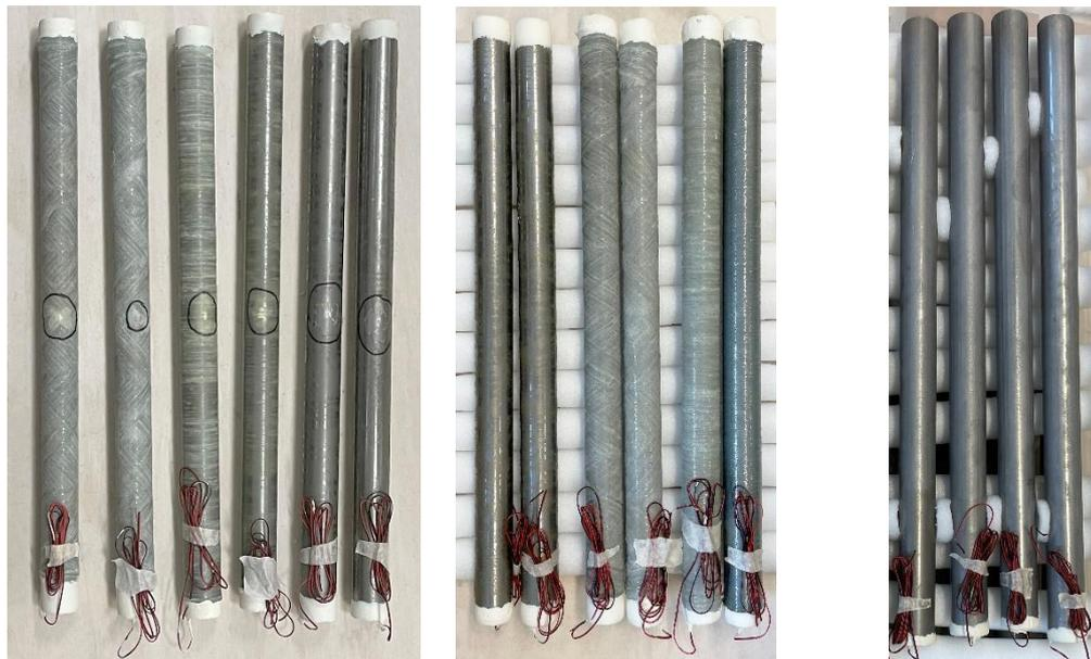
(a) Impacted specimens      (b) Intact specimens      (c) Uncoated specimens
