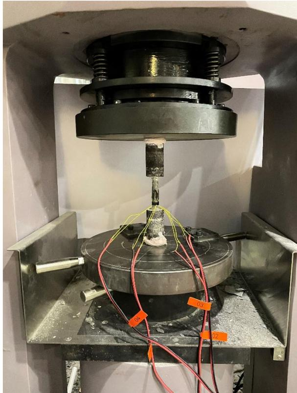
(b) Setup for compressive tests
