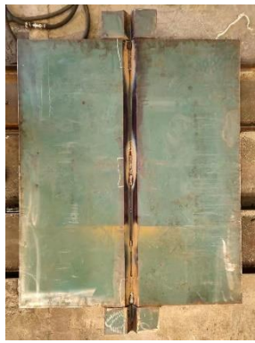
a) Welding of run-on plate
