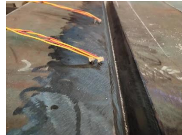
c) Thermocouples were spot welded
