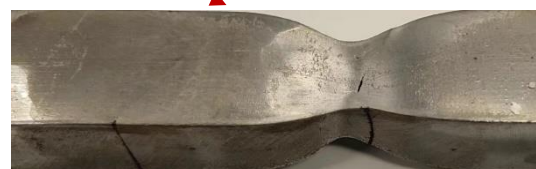
Fractured at HAZ
