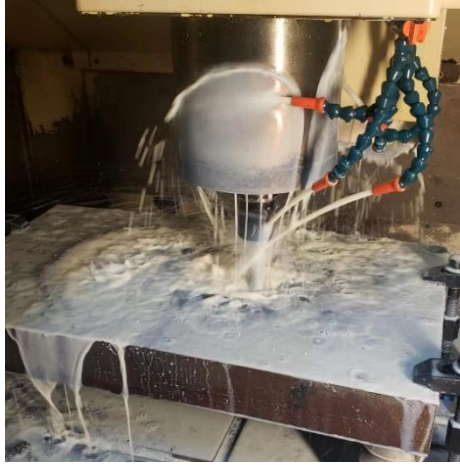
a) Milling for material removal b) Hole-drilling on the newly formed surface
