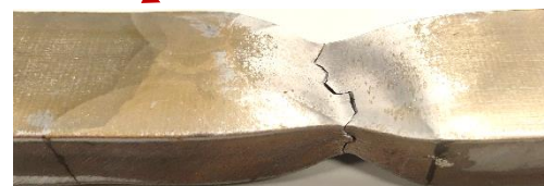
Fractured at HAZ
