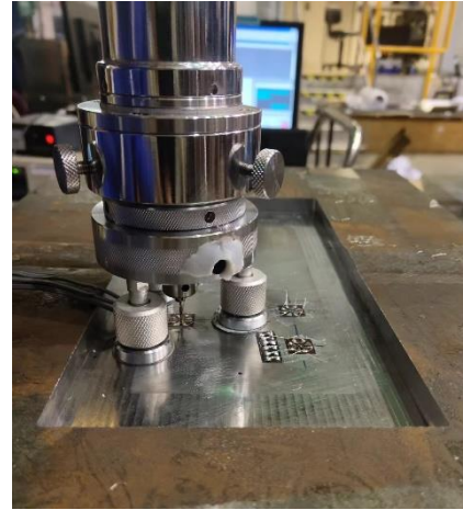
a) Milling for material removal b) Hole-drilling on the newly formed surface
