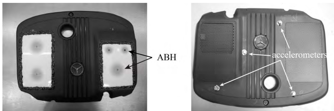
Fig 1.9 ABH engine cover (top view) and location of accelerometers on reference engine cover [52].
