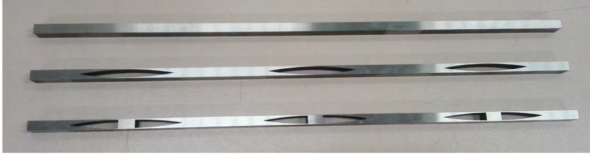
Fig 1.12 Uniform beam (top), beam with periodic ABH elements without studs (middle), beam with periodic ABH elements with studs (bottom). [25]
