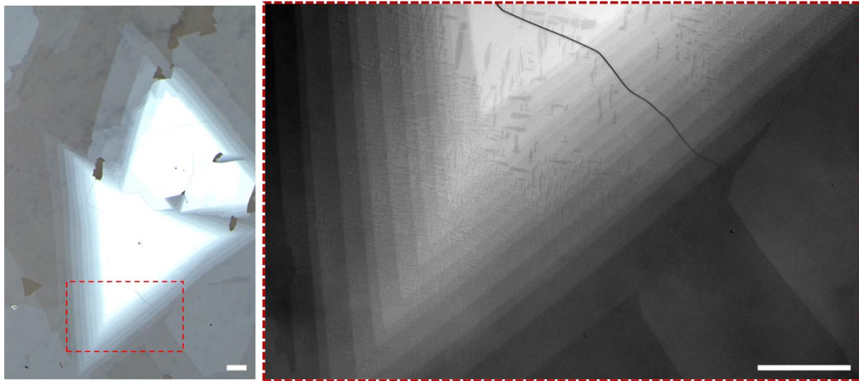
Figure 3.8 Polarized optical microscopy of as growth sample with cracking inducing phase transition. The scale bar is 40 \mu\text{m} .
