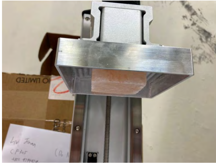
Figure 5-2. Fabrication of AFMSs and samples: the modified building plate before photolithography, which is a rectangular cavity adhered with a salt brick.
