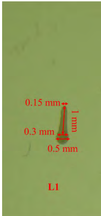
Figure 5-4. Dimensions of AFMSs and the material sample: the dimensions of AFMS L1, which is around 1 mm long and 0.3 mm thick.
