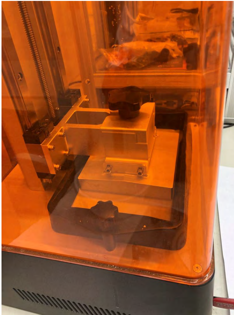
Figure 5-1. Fabrication of AFMSs and samples: the 3D printer for photolithography with photosensitive resin inside its vat, and the building plate is immersed in the resin.
