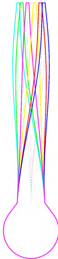
Figure 3-31. The combination of the profiles at a head amplitude equal to 12 μm for the parameters the same as \lambda = 0.9 in Figure 3-30.
