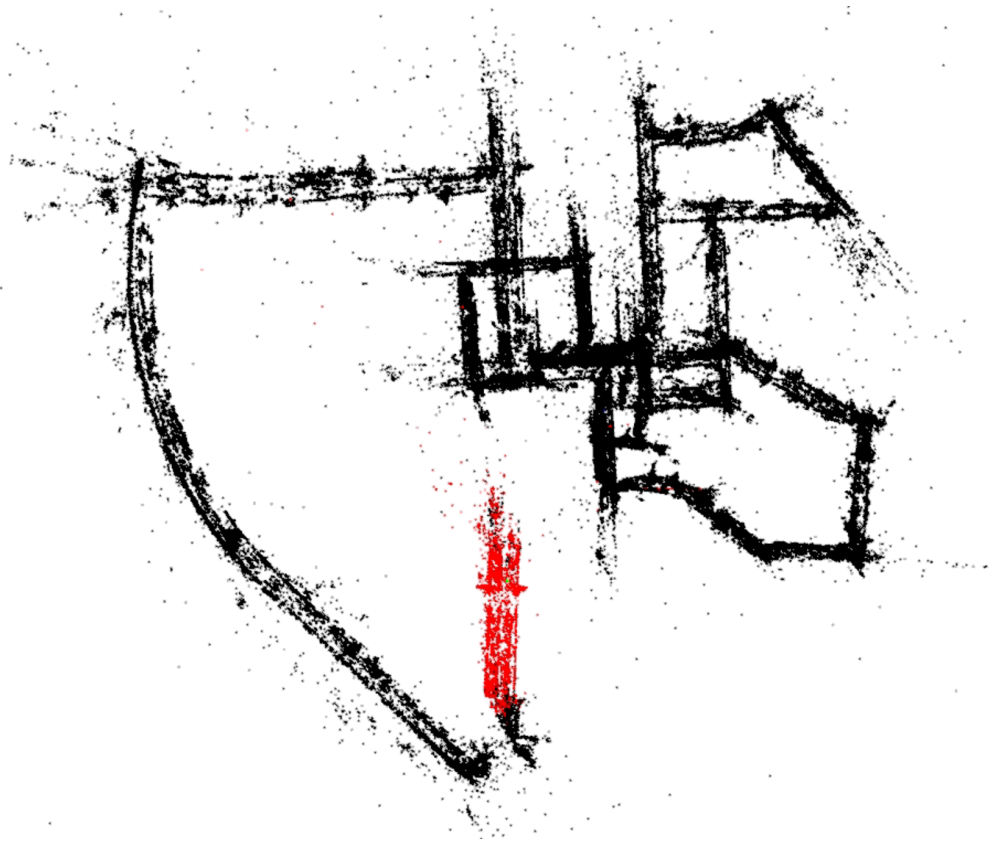
Figure 7. Feature point map of sequence 00 in KITTI odometry dataset [63] constructed by ORB-SLAM 3 [45]
