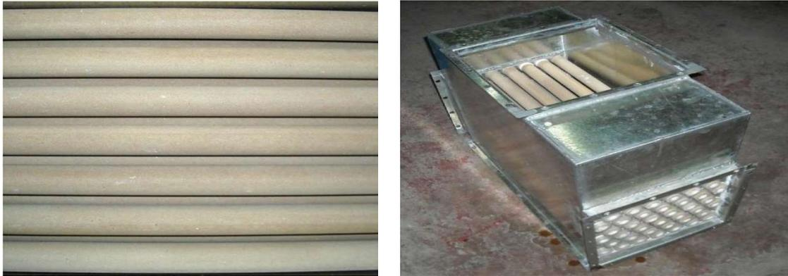
Fig. 2.2 Schematics diagram of tubular type IEC
