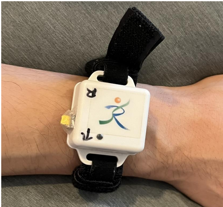
Figure 6-2: Sham device (standard accelerometer)
