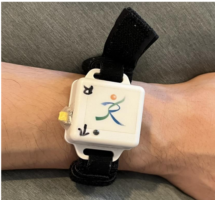
Figure 6-2: Sham device (standard accelerometer)
