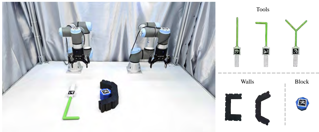
Figure 5.1: Tool-Object manipulation in a dual-arm robotics system with environmental constraints using the non-prehensile approach.
