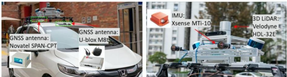
Figure 3.4 Experimental setup of the LiDAR. a dataset for the evaluation of multi-vehicle cooperative SLAM.
