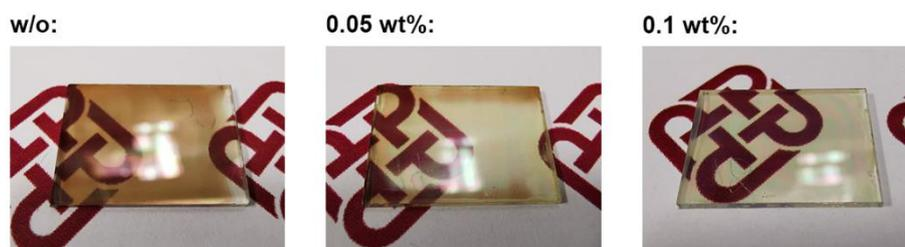
Figure 3. 3 Photographs of the as-cast perovskite films with different amounts of TAH before thermal annealing.
