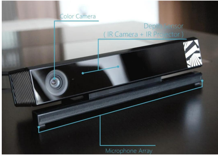
Figure 3.15: Structure of Kinect2 .
