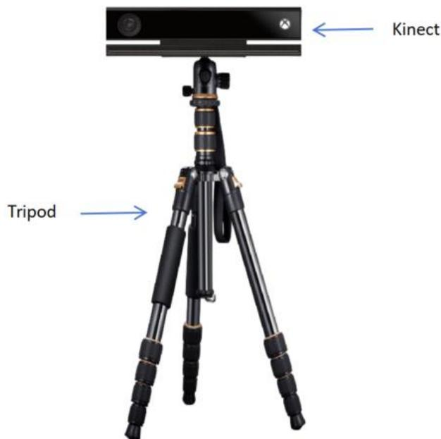
Figure 3.14: Hardware composition of system.
