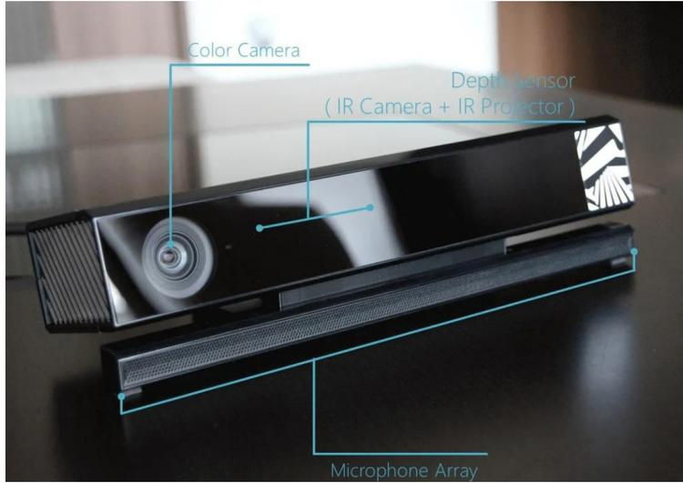
Figure 3.15: Structure of *Kinect2*.
