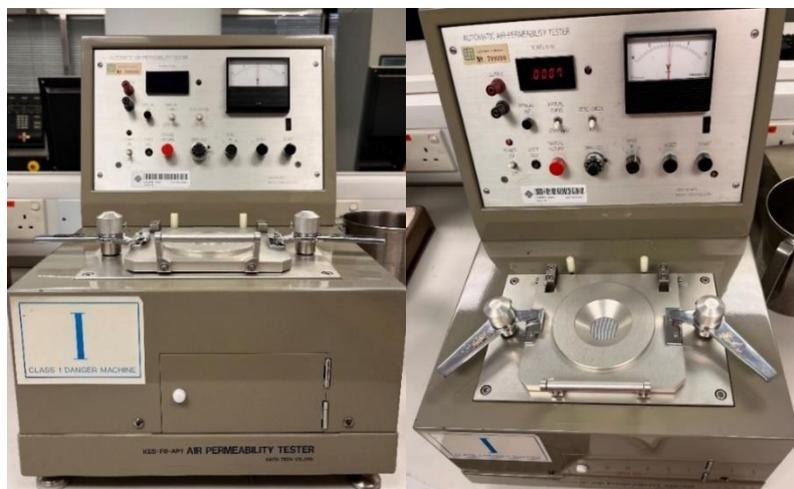
Figure 3.10 KES-F8 Air Permeability Tester
