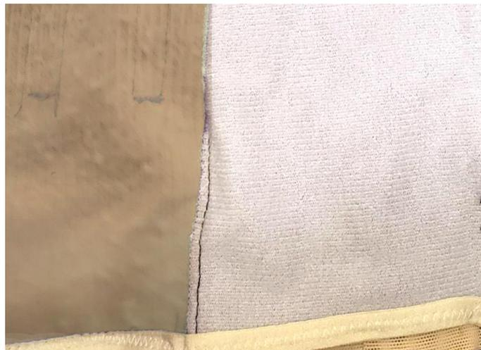
Figure 3.6 Pilling on tricot fabric of original design
