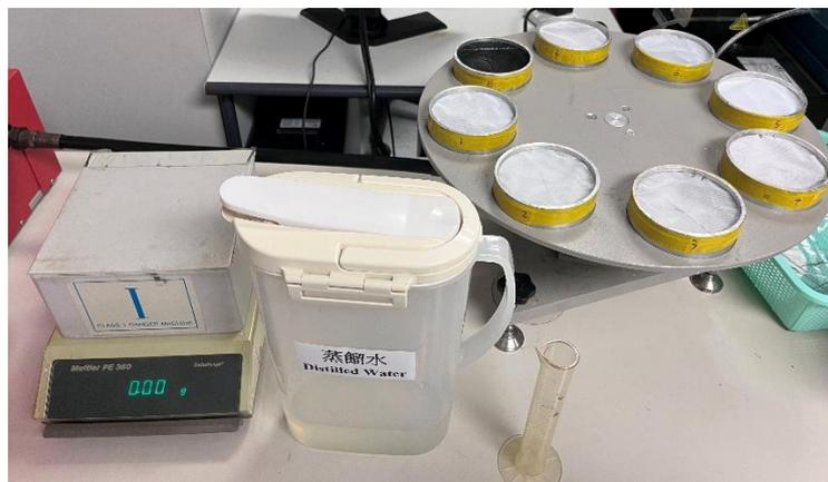
Figure 3.11 Set up of water vapor permeability test
