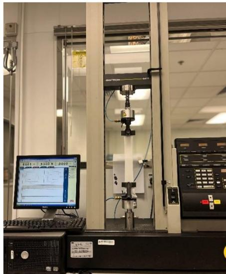
Figure 3.8 Instron 4411 tensile strength tester
