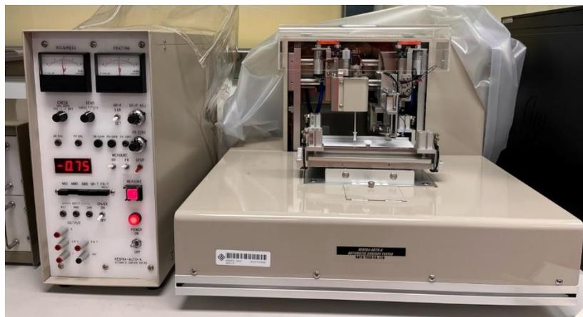
Figure 3.14 KESFB4-AUTO-A Automatic Surface Tester
