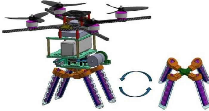
Figure 1.1: Prototype of the proposed soft aerial vehicle (with H-base soft gripper (left) or X-base soft gripper (right)).
