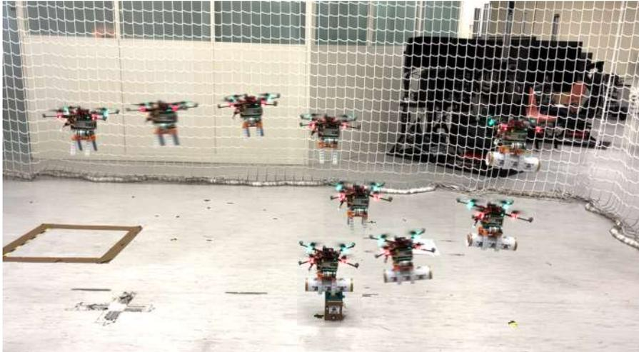
(a) grasping a shuttlecock tube with 46 g load.
