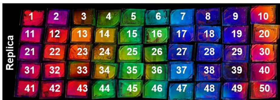
Figure 4.10 Optical images of 50 replica samples of the Cu grating pattern fabricated by the same Au template under the emission of light.
