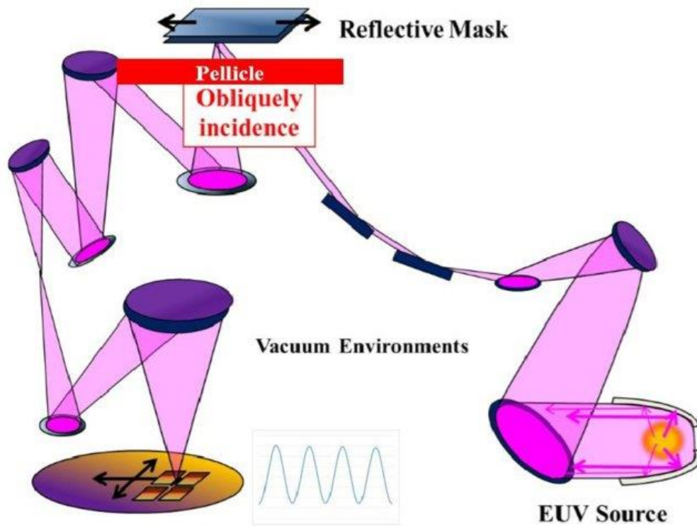
Figure 2.5 Schematic presentation of the function mechanism of EUV lithography[81].
