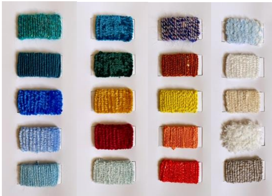
Figure 4.11 Electronic yarns using 210D PE core yarn and concept B cover yarn
