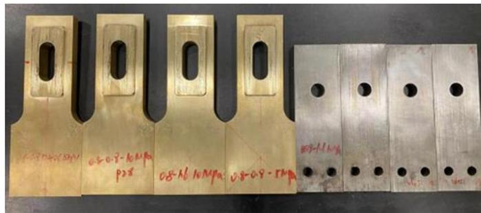
Fig. 4.9 Surface wears after friction tests
