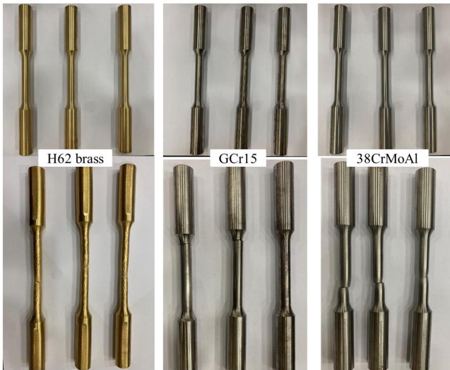
Fig. 4.1 Material coupons before and after tests
