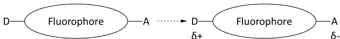
Figure 1.5: Dipole moment increases when excitation of ICT systems.
