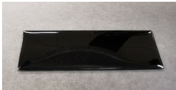
Figure 6.7 Glass slide coated with asphalt binder for contact angle test
