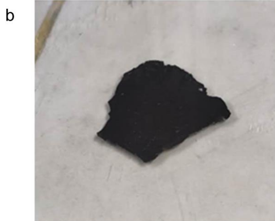
Figure 4.5 (a) XRD patterns of pristine \text{LiMn}_2\text{O}_4 , the free-standing electrode (FS-LMO), and FS- \text{Li}_{1-x}\text{MO} (b) A digital image of the free-standing FS-LMO electrode.
