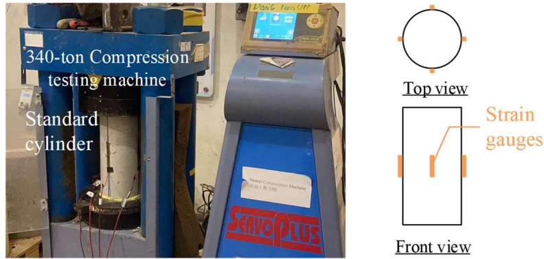
Figure 6.11 Standard static tests for the modulus of elasticity
