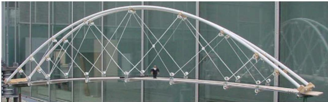
Figure 2.8 Scaled model of FRP self-stressed bowstring footbridge (Caron et al., 2009)
