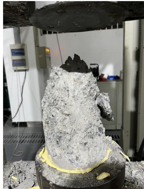
(b) Typical failure mode
