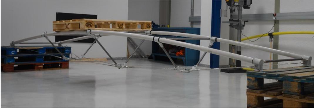
Figure 2.9 Prototype of bending-active tied footbridge (Bessini et al., 2019)
