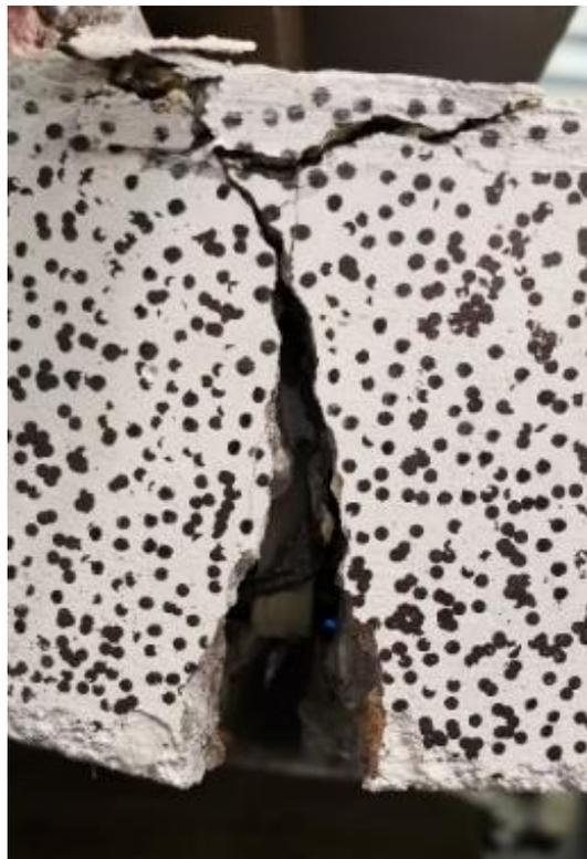
Figure 3.5 Fracture of concrete near the arch crown at the failure point
