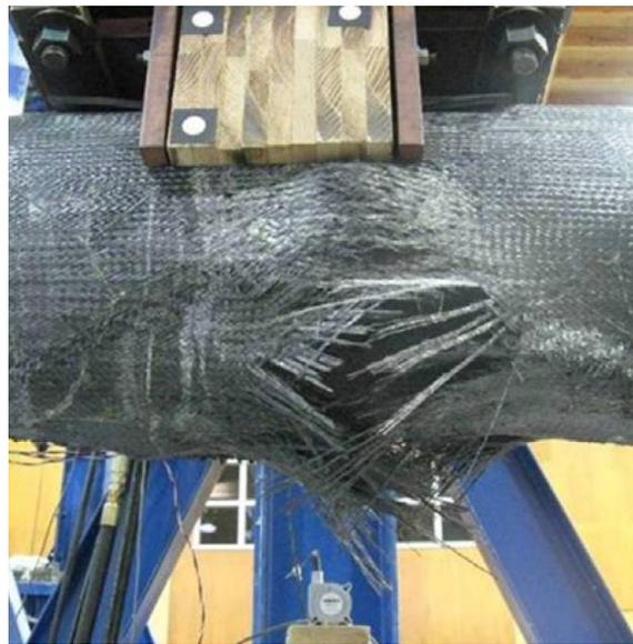
(b) Typical failure mode
