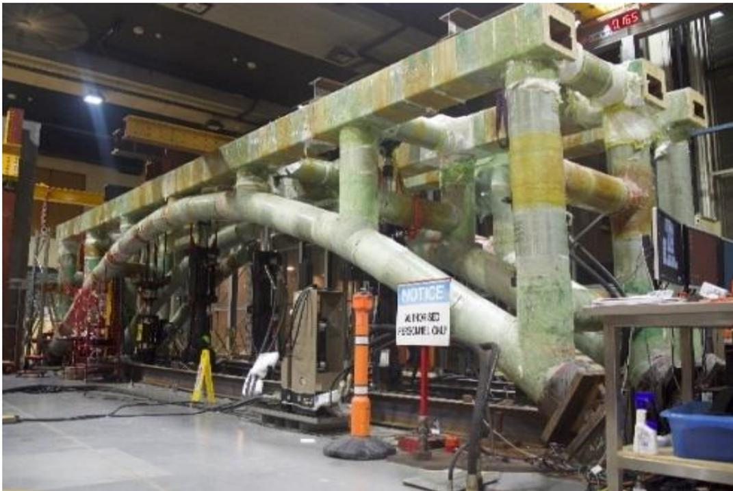
Figure 2.15 DSTA bridge constructed at University of Queensland, Australia (Burnton et al., 2019)
