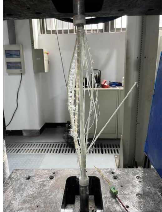
(b) Typical failure mode
