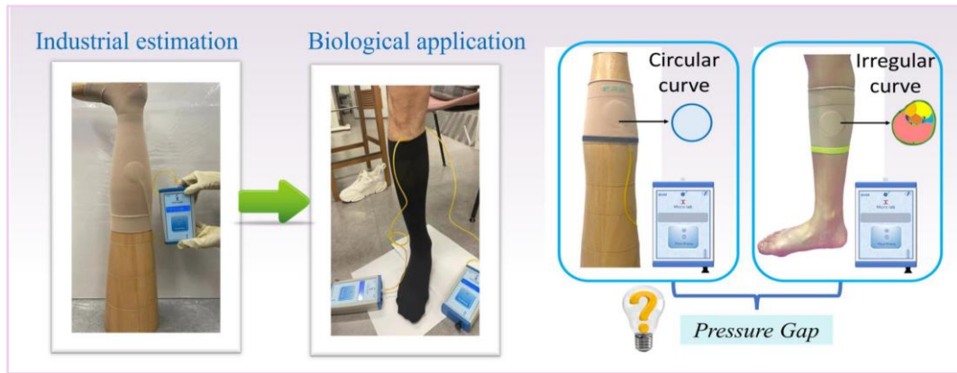
Figure 2.10 Pressure evaluation by leg model and practical use by bio-leg.
