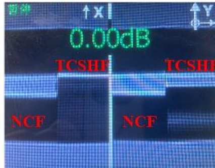
Fig. 4.4 The microscope image of the fusion splicing point between NCF and TCSHF
