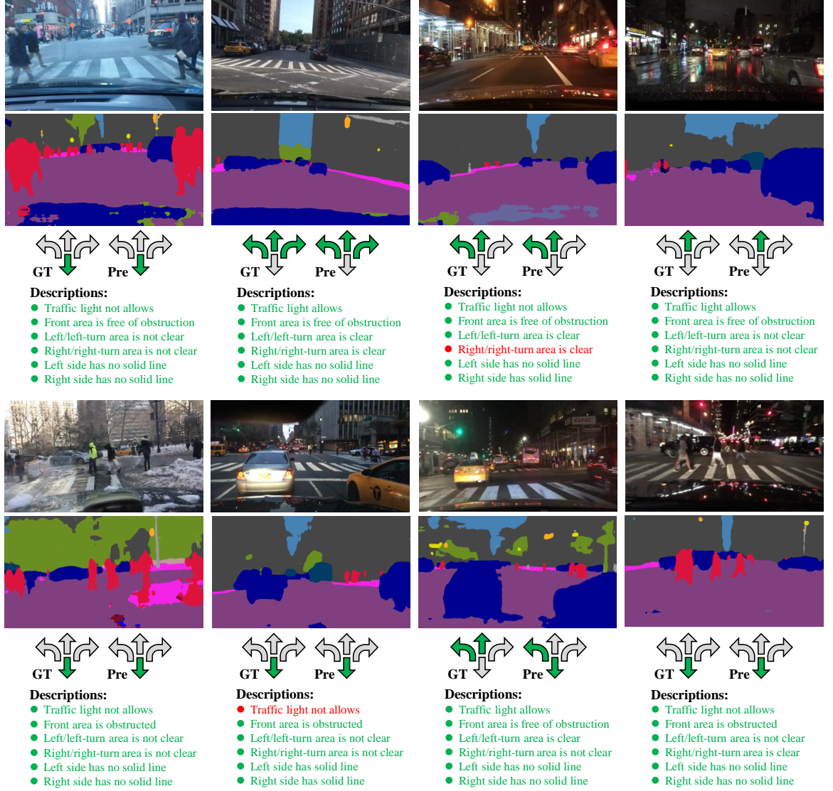
Figure 3.4: The sample prediction results of the decision-making actions and the surrounding environment descriptions of the ego-vehicle.
