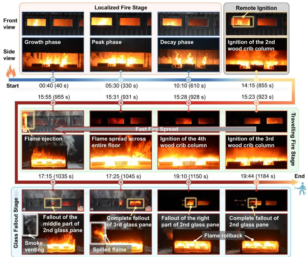
Fig. 5.3 Timeline of the Test A without ‘active opening’ strategy.
