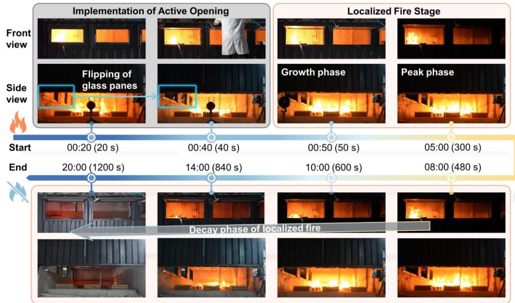
Fig. 5.4 Timeline of the Test B with ‘active opening’ strategy.
