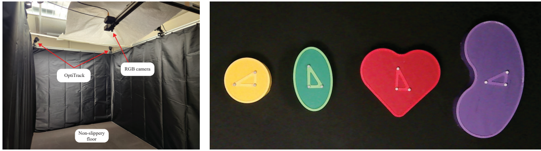
Figure 6.2: Left: Experimental platform. Right: Manipulandums of 4 different shapes: circle (yellow), ellipse (green), heart (red), bean (purple).
