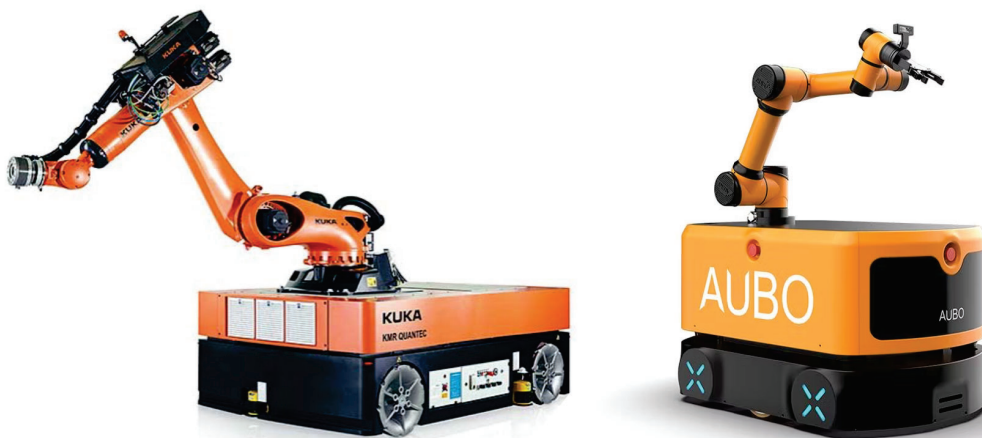
Figure 1.3: Examples of conventional mobile manipulators. Left: KUKA KMR QUANTEC. Right: Aubo Robotics AMR300.
