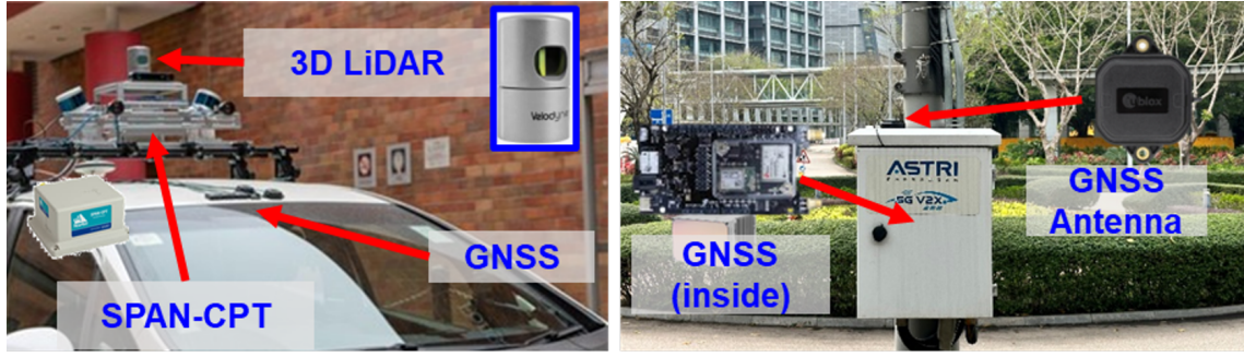
Figure 6.16: (left) Sensor setup for the onboard and RSG platform. A u-blox F9P GNSS, Velodyne 3D LiDAR, Xsens MTi-10 IMU, and SPAN-CPT for the onboard while two u-blox GNSS are connected with different roadside infrastructures; (right) U-blox GNSS is integrated with each roadside infrastructure.
