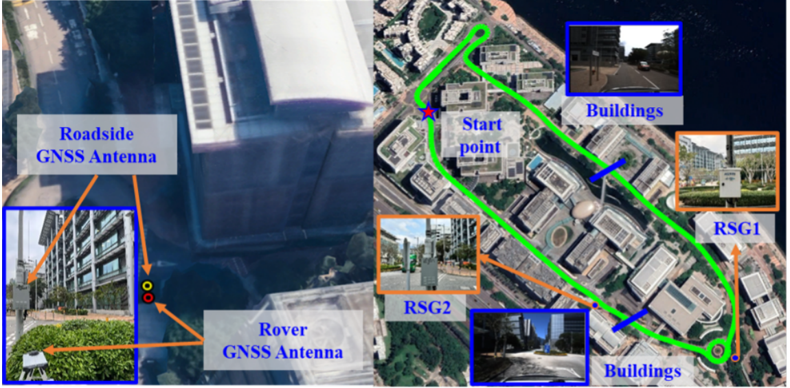
Figure 6.15: (left) The static experiment near a tall building using one RSG and one rover GNSS compared with the traditional open-sky base station (baseline: 4.34 km) and one rover GNSS (short baseline: 2.26 m); (right) The dynamic experiment in Hong Kong C-V2X testbed which contains multiple RSGs and the evaluated ground truth trajectory.
