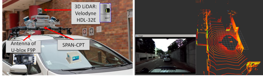
Figure 5.3: Left: Setup of the sensor platform, which includes a u-blox F9P receiver, Velodyne HDL-32E 3D LiDAR, and ground truth positioning provided by the SPAN-CPT. Right: A typical urban environment in Hong Kong for evaluation.
