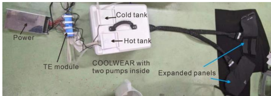
Figure 3.12 Temperature maintenance ability experimental set up of thermoelectric (TE) module by attaching to COOLWEAR system.
