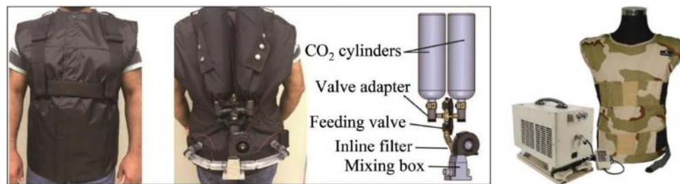
Figure 2.10 Front view, back view, and the air treatment system of the cooling garment [132,133].
