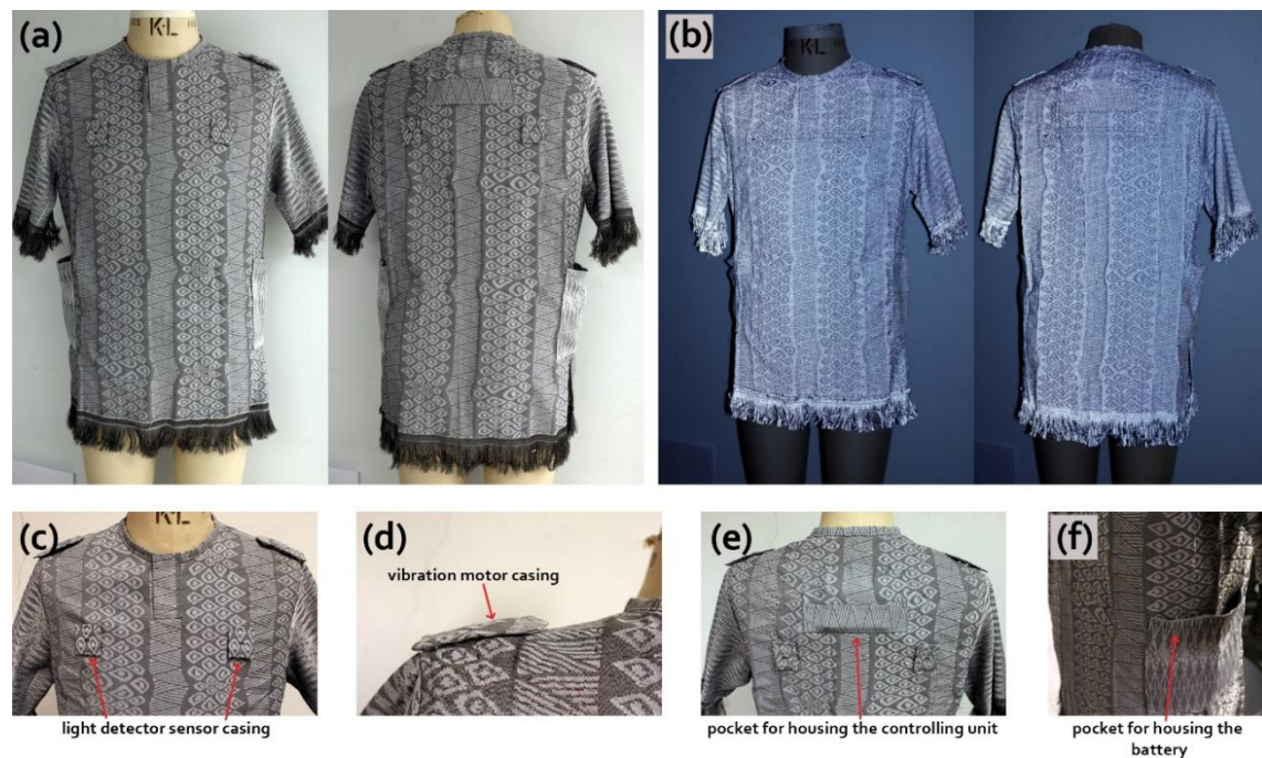
Figure 5.33. Assembled components on the jacquard retro-reflective woven fabrics. (a) the appearance of the assembled components on the front and back bodice, (b) reflective effects in the darkroom setting taken by a digital camera, (c) and (d) positioning of the light detector sensor and vibration motor, (e) positioning of the controlling unit at the upper side of the back bodice, (f) pocket for housing the batter pack to power the microcontroller.
