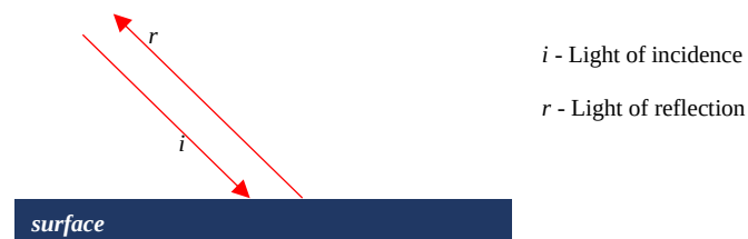
Figure 2.6. Principle of retro-reflection
