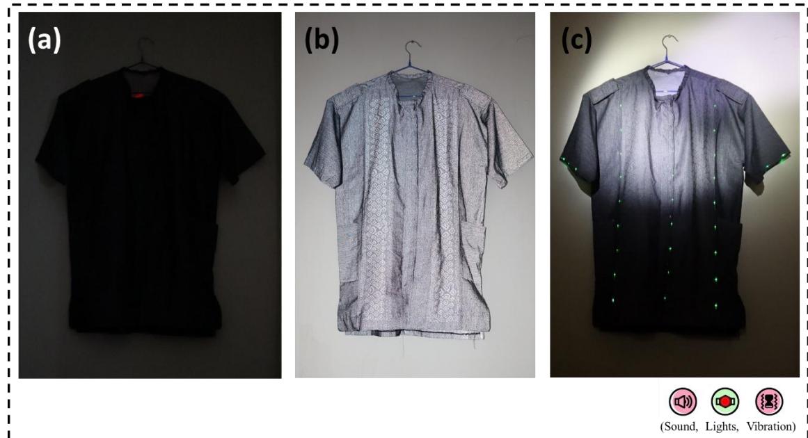
Figure 5.42. (a) Appearance of the assembled clothing with no lighting effects in the darkroom setting. (b) retro-reflective effects in the darkroom setting. (c) lighting effects of the green LEDs when light is detected in the darkroom conditions at the laboratory.
