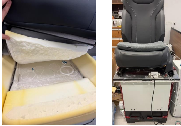
Fig. 4.8. (a) The main sensor placed in the seat, (b) system setup.
