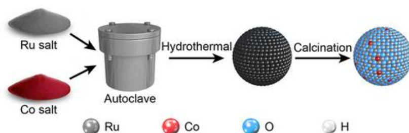
Figure 1.6. A schematic illustration of the synthesis process of the Co single-atom-incorporated RuO 2 sphere. [90]
