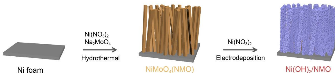
Figure 5.1. A schematic diagram of the synthetic procedure for Ni(OH) 2 /NMO.
