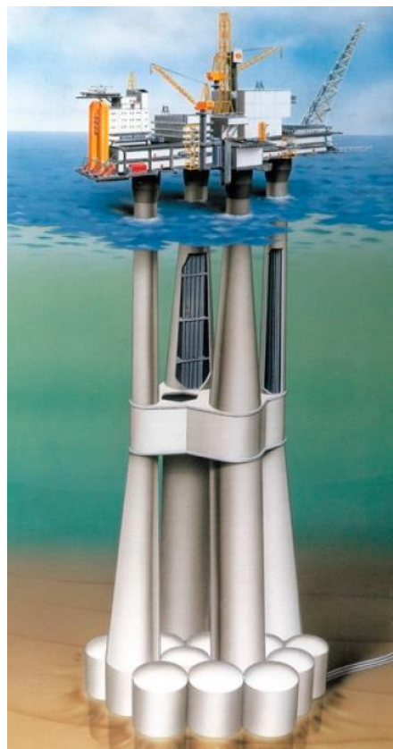
Fig. 2.3 An illustration of Condeep oil storage platform (source: Galbraith et al. 1993)
