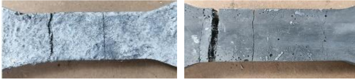
Fig. 3.4. Typical crack patterns observed in specimens under static and fatigue loading conditions
