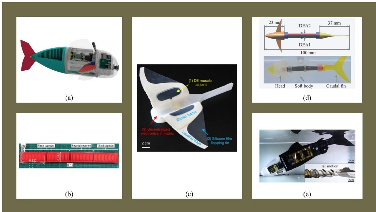
Fig. 2.3: Soft swimming robots. (a) Robotic fish SoFi. (b) Soft robot eel. (c) Pressure-resilient soft robot fish (d) Bionic muscle actuated soft robotic fish. (e) Untethered artificial fish.
