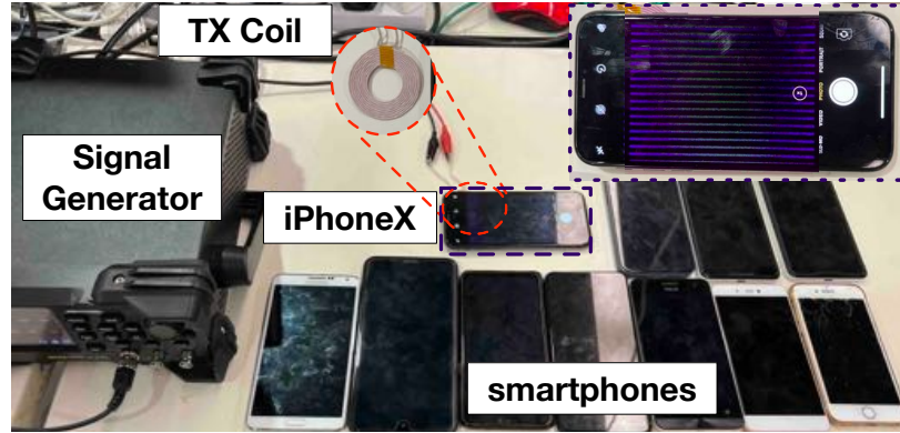
Fig. 4.4: Experimental setup for the real-life feasibility verification.
