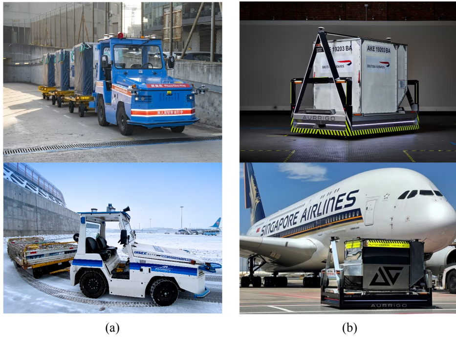
Figure 1.2: Airport baggage transport vehicles: (a). tractor and trailers; (b). electric auto-dolly.
