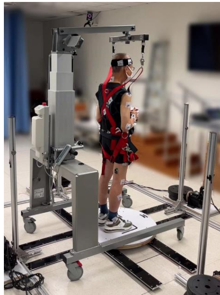
Figure 4-1. The moving-platform perturbation system with the subject.
