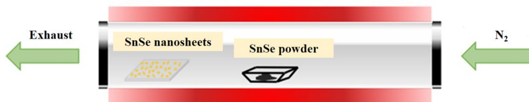
Figure 3.3 The vapor transport deposition setup for SnSe nanosheets growth.
