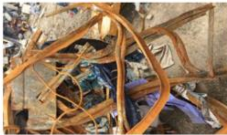
(b) Parts of distorted Vierendeel beam parts found in the debris.
