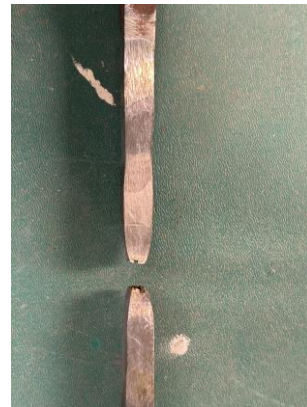
(b) Fracture at HAZ/BM interface: Q690-B6-H1-2
