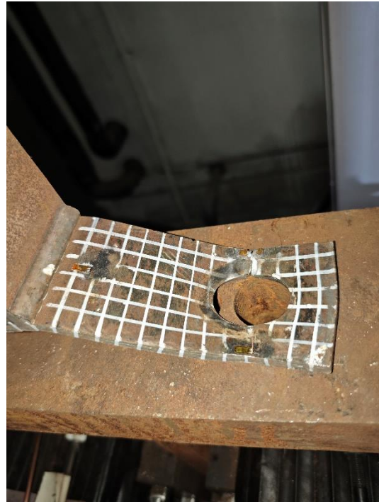
(b) Q460-H3-E40-Rig, bolt hole failure
