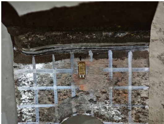
(a) Q960-H1r-E80-Rig, 0.547 kJ/mm
