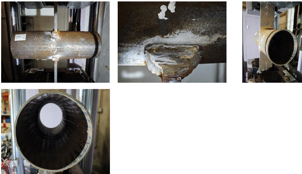
Figure 6.13 Experimental failure mode of No.2-4C200x6*-XT-B-Tran-0_7-M
