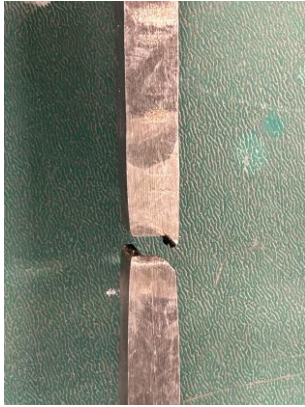
(c) Fracture at HAZ: Q960-B6-H1-2
