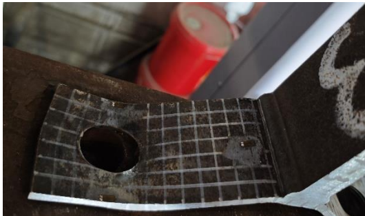
(c) Q460-H3-E40-Rig, 1.267 kJ/mm
