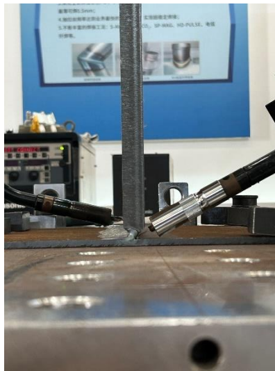
Figure 4.10 Welding angle and placement of welding gun
