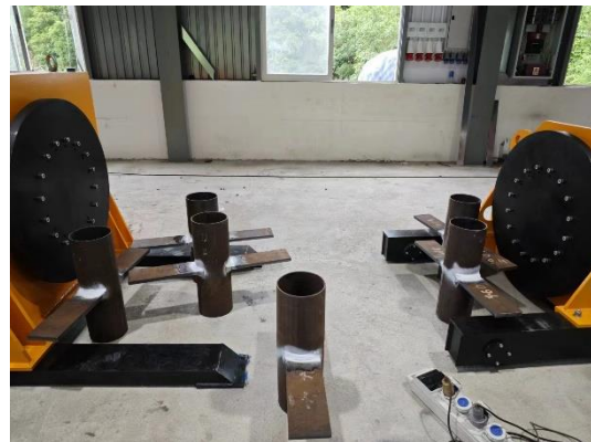
Figure 6.5 The completed gusset plate to CHS X-joints
