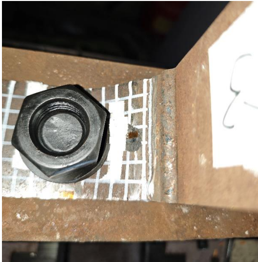
(c) Q690-H3-E80-Rig, 1.126 kJ/mm
