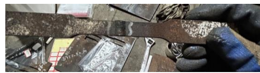
Figure 3.4 Butt-welded tensile coupons cut from butt-welded joints
