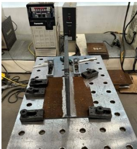
Figure 4.5 Prevention of welding distortion
