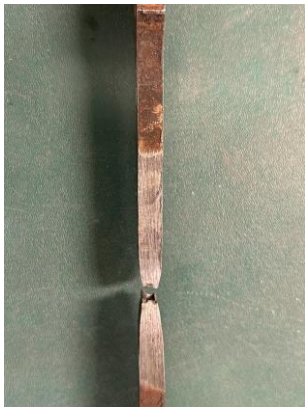
(a) Fracture at BM: Q460-B6-H1-1
