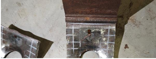
(a) Q460-H1-E80-Rig, 0.531 kJ/mm
