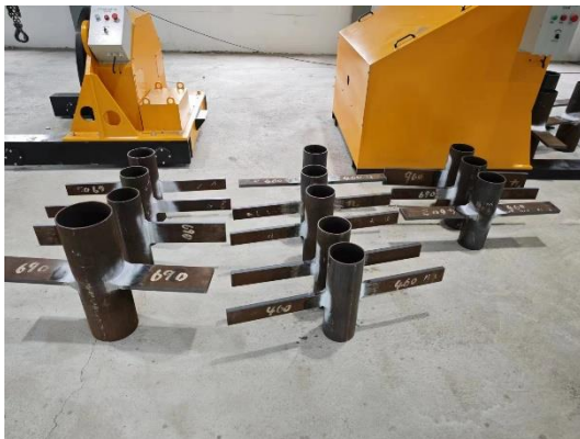
Figure 6.5 The completed gusset plate to CHS X-joints
