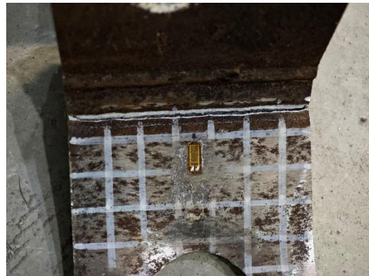
(b) Q960-H2r-E80-Rig, 0.775 kJ/mm
