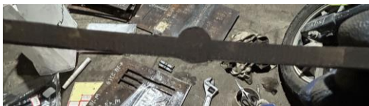
Figure 3.4 Butt-welded tensile coupons cut from butt-welded joints
