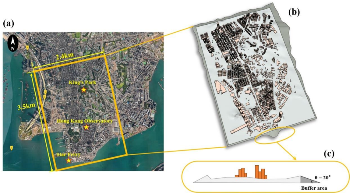
Fig. 4.6 Study area for CityFFD simulation: (a) plane view of the target area (where weather stations are marked with stars), (b) geometries of buildings and terrain, (c) setting of buffer areas.
