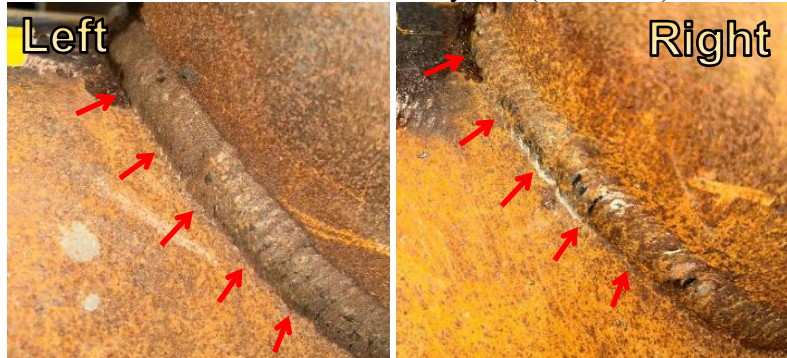
Crack initiation at cycle 2
