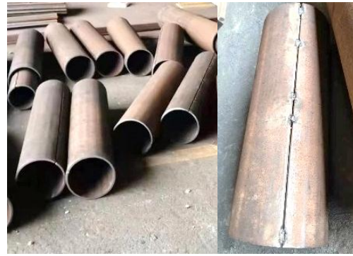
b) Cold-bent steel tubes with tack welds
