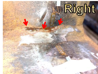
Crack initiation at cycle 1
