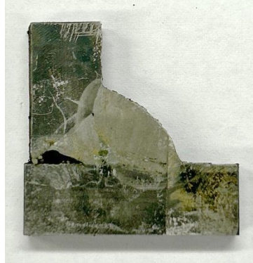
Joint CT5: Fractured part R
