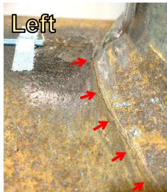
Crack initiation at cycle 310
