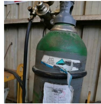
c) Shield gas: 20% Ar + 80% \text{CO}_2
