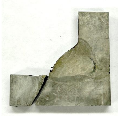
Joint CT5: Fractured part L
