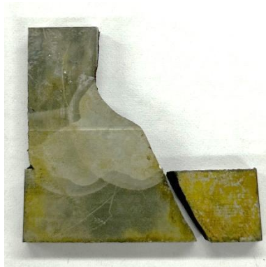
Joint CT3: Fractured part R
