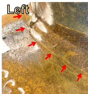
Obvious crack growth at cycle 325
