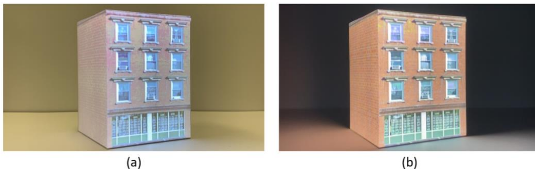
Figure 3-4 Comparison of projection results with illumination condition. (a) Projection with environmental electric light; (b) Projection without environmental light
