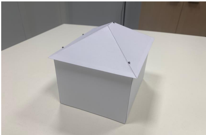
Figure 5-7 building prototype with hemispherical reflective markers
