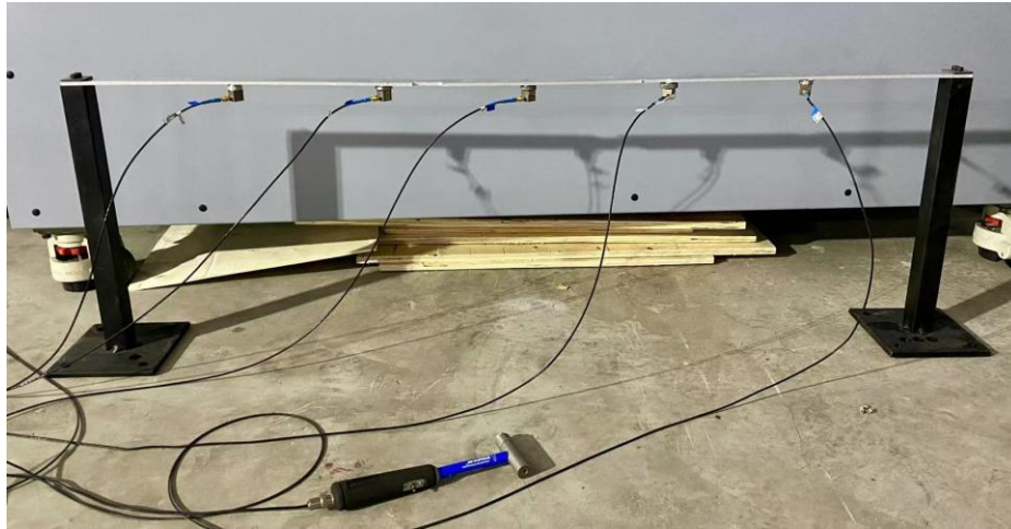
Figure 6.22 Vibration test of aluminum beam
