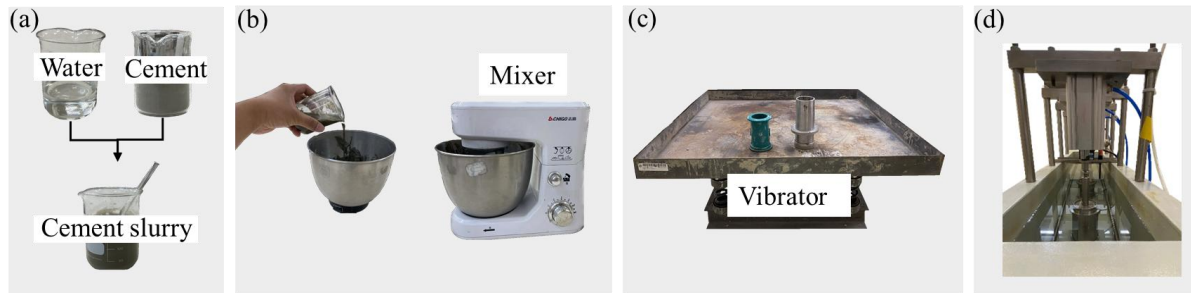
Figure 3.2 Photographs showing the specimen preparation process: (a) cement slurry preparation; (b) mixing of marine clay and cement slurry; (c) specimen preparation using vibrator; (d) curing of specimens in curing machine.
