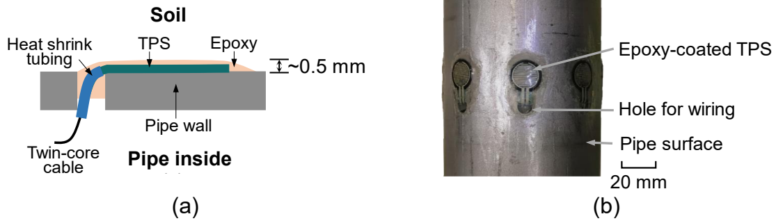
Figure 3.8 Design of TPS-based ICPT sensors: (a) schematic side view; (b) photograph
