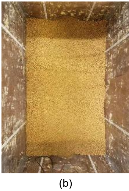
Figure 3.25 Model preparation of CDG: (a) sieve; (b) soil before compaction; (c) electric earth rammer
