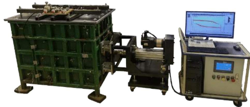
Figure 3.1 Experiment system for ASPI physical modelling tests: (a) schematic diagram; (b) photograph
