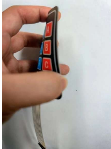
Figure 4-3. Deformation of the membrane keypad.
