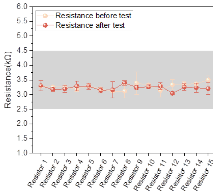
Figure 4-17. Resistance difference between keys before, and after the cyclic temperature test.
