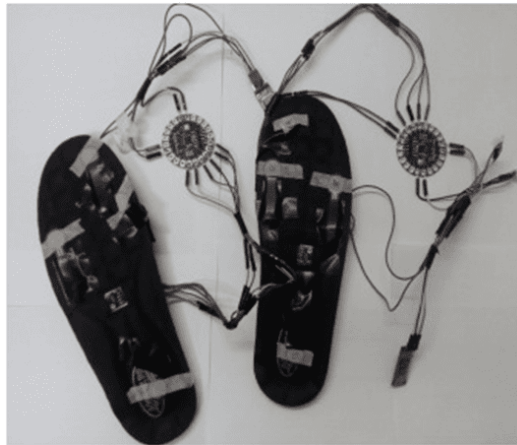
Figure 2-12. Designed insole system for diabetic foot.
