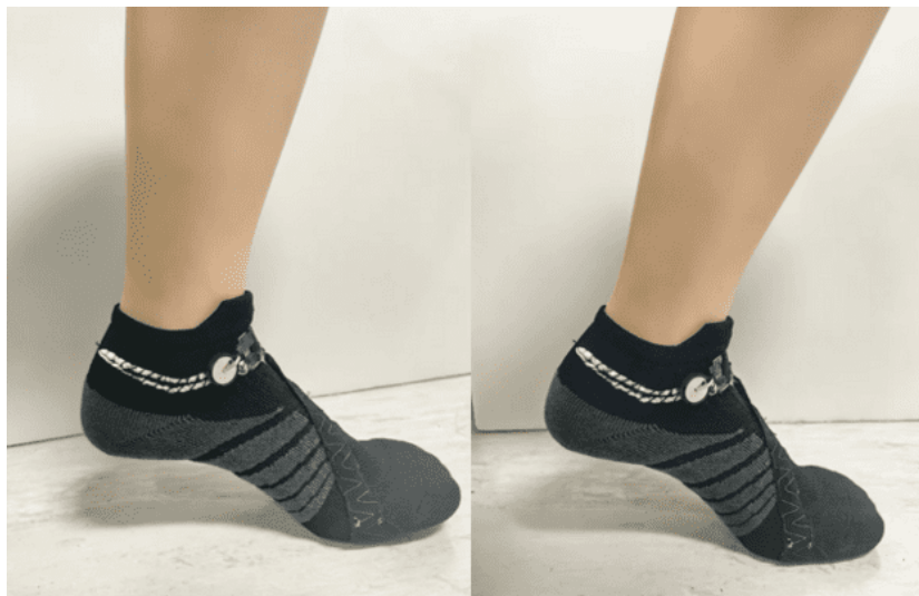
Figure 5-21. Mannequin wearing the sock for diabetic patients. Left: LED is in off-state. Right: LED is in on-state.
