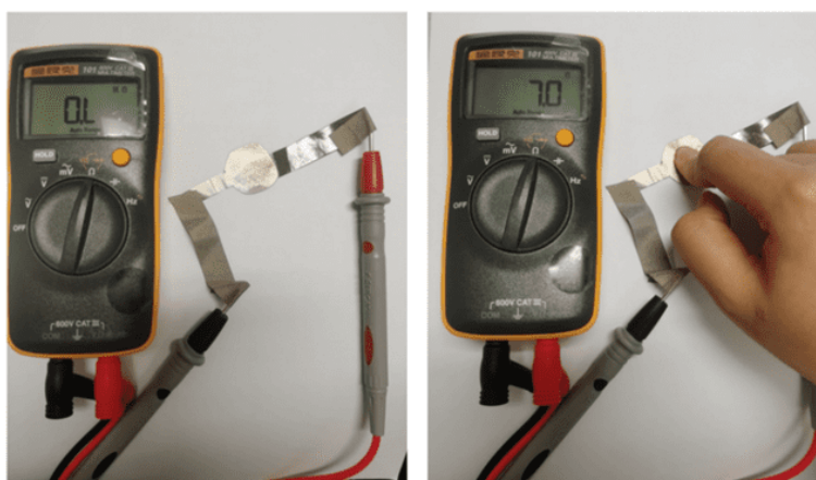
Figure 3-3. Image of the fabric-based mechanoreceptor on-off resistance.
