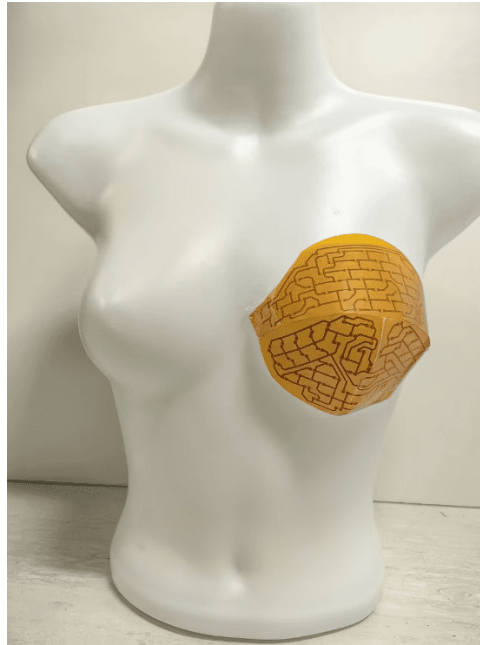
Figure 7-22. Conformability of the flexible PBM panel
