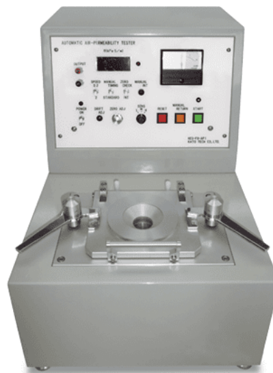
Figure 6-4. Photo of the KES-F8 air permeability tester.
