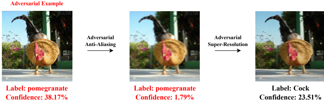
Figure 6.1: The proposed adversarial defense pipeline. We give an adversarial example of “cock” class with AutoAttack \ell_{\text{inf}} = 8/255 on ImageNet dataset. Adversarial anti-aliasing aims to eliminate adversarial perturbations, while adversarial super-resolution seeks to restore benign images from blurred adversarial examples using prior knowledge from the clean dataset.
