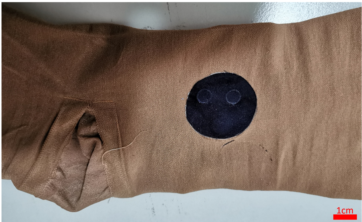
Figure 3-4 The compression garment with a flexible pressure capacitive sensor.
