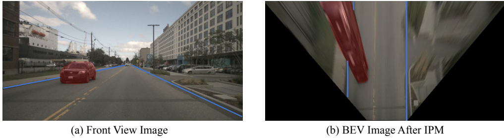
Figure 4.5: The front-view image of the road and that in bird-eye view after IPM
